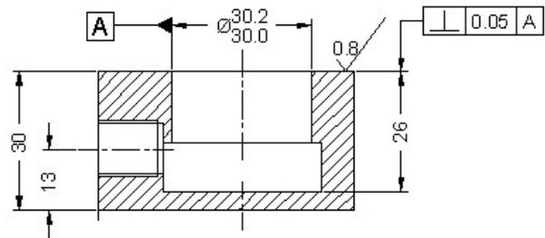
All dimensions are in mm, Overall dimension tolerance  $\pm 0.5$  mm.
